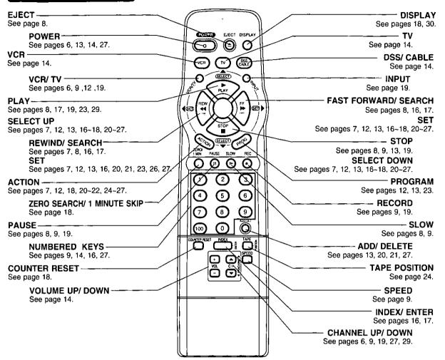
**EJECT button:** When EJECT is pressed, the tape is ejected from Cassette Compartment. If EJECT is pressed during recording, the VCR will not respond to the command.
